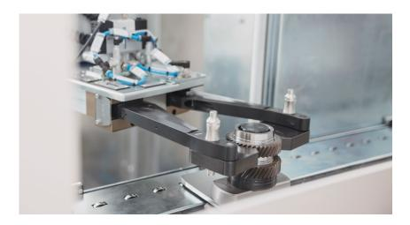
enable a changeover process in less than ten minutes without requiring tools. Teaching new, non-stored workpieces takes about 20 minutes. This simple and time-saving operation is also appreciated by the personnel, who are trained in all the important functions of the loader in less than two hours.
