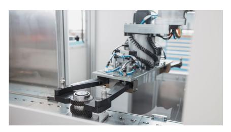
grams enable a changeover process in less than ten minutes without requiring tools. Teaching new, non-stored workpieces takes about 20 minutes. This simple and time-saving operation is also appreciated by the personnel, who are trained in all the important functions of the loader in less than two hours.
